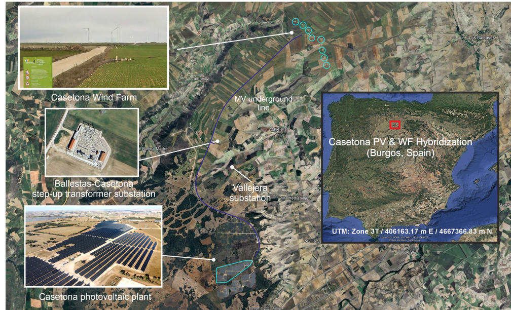
Figure 3. Location of the Casetona WF-PV Hybridization Project. Red box shows the location of the hybrid power plant in Spain. Blue circles show the location of the WTs, red box shows the Own elaboration.
